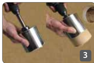
3 Push out the drill core with the aid of the ejection system
