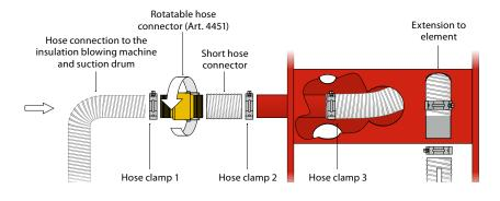
The rotatable hose connector allows full use of the hose reel and enables the insulationblowing team to achieve optimal site efficiency.
