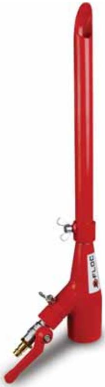
Spray head with inline nozzle for injection and adhesion of EPS granules. A complete wetting of the EPS beads enables a permanent solidification of the hollow layers insulation after the adhesive has been hardened. Settlements, material trickling out through gaps and cracks or subsequent changes can therefore not occur. The thin-walled nozzle pipe with its special shaped outlet enables a high processing speed at a relatively small bore diameter.
