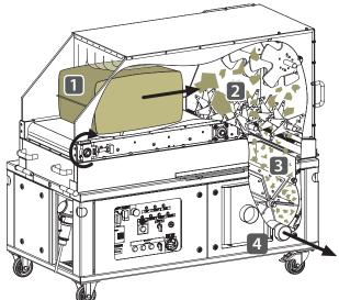
1 The insulation bales are conveyed via the conveyor belt into the hopper.
