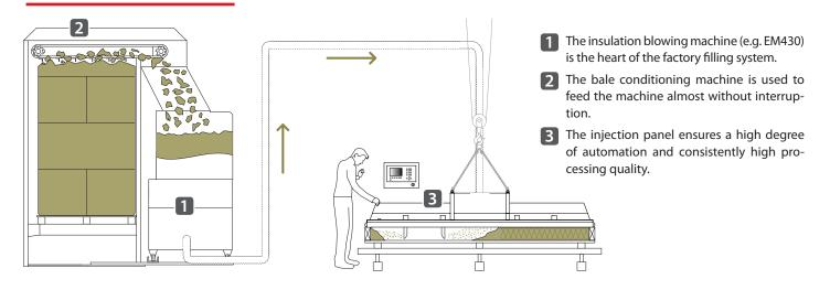
The factory filling systems are designed so that different insulation materials (see: Blow-in insulation material product groups) can be used. Typical product classes such as wood fibre, cellulose, glass wool and rock wool have already been extensively tested.
