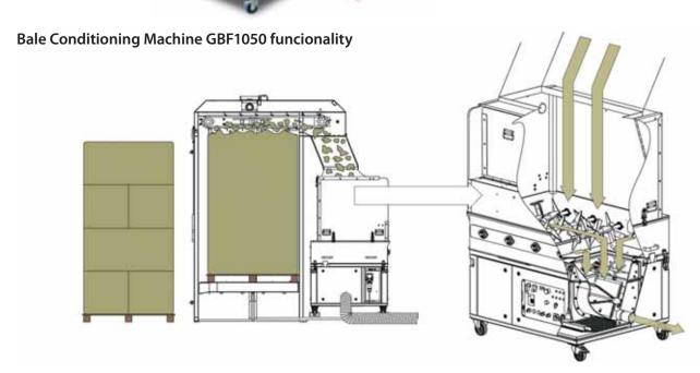
The Bale Conditioning Machine GBF1050 is specifically designed for the bale conditioning processing of insulation materials or stacked insulation bales. The machine is intended for stationary use, where it forms the base for a highly efficient filling for wall, ceiling and finished elements.
