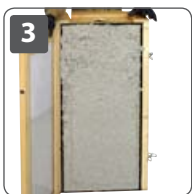
Opening the test element to examine the filling results.
