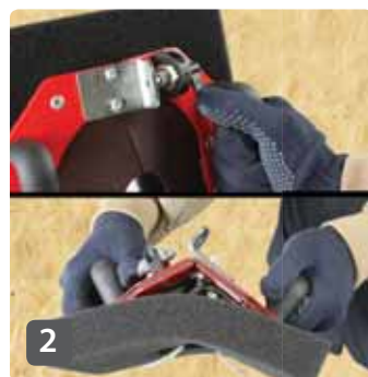
2 Open the locking latch and fold in the hose bushing
