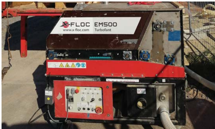
The high-performance blow-in machine X-Floc Turboblast EM500...
