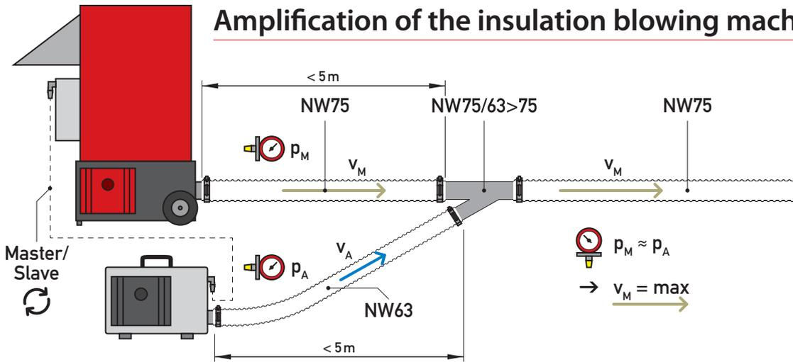
The insulation blowing machines' air power can be optimized by using an amplifier/vacuum station. For an effective and trouble-free performance increase of a blowing machine by means of amplifier/extraction technology, the following principles must be observed:
